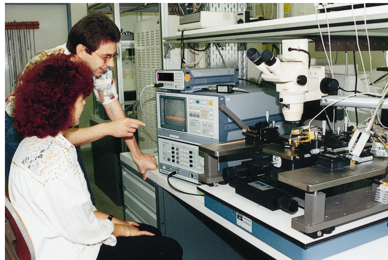
FIG 2 On-wafer test setup for noise measure- ments with Spectrum Analyzer FSM at Ferdinand Braun Institut für Höchstfrequenz- technik, Berlin Photo: Blask
